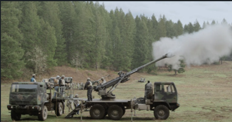
BRUTUS 155MM MHS (MOBILE HOWITZER SYSTEM) CONCEPT
